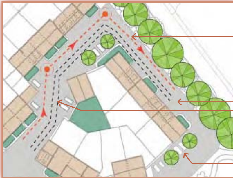
Figure 19: The road design incorporates service strip and sewer.
