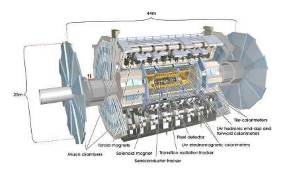
This is a cutaway drawing of the ATLAS detector showing the beam pipes at either end. The central parts, the Pixel Detector and Transition Radiation Tracker measure the paths of the charged particles. The next section has the calorimeter devices which measure the energies of particles and after this is the muon spectrometer which measures the tracks of muon particles.
