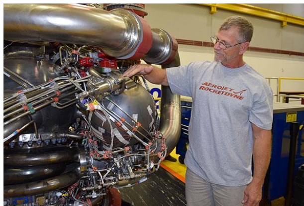
An Aerojet Rocketdyne technician inspects the 3-D printed pogo accumulator assembly on an RS-25 development engine at the Aerojet Rocketdyne facility located at NASA's Stennis Space Center
