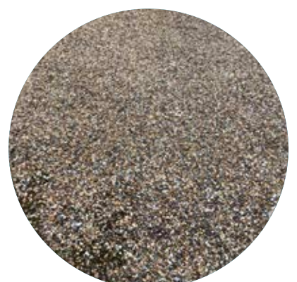
GRAVELS AS POROUS SURFACE MATERIAL
