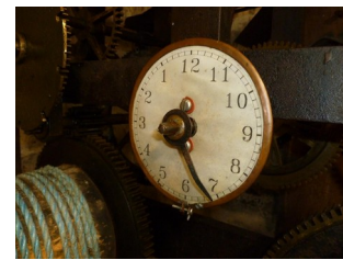
The right weight drives the train and the left weight drives the striking mechanism
