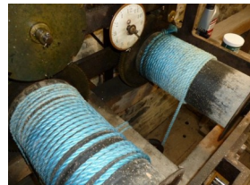
Drums of rope that support the weights
