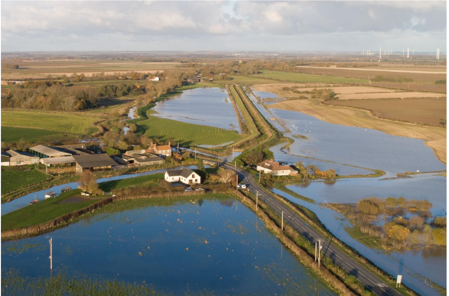
Photo courtesy Mike Hopps, Drifffield & Wolds Weekly. The Old Howe, empty because it has been blocked off rather than repaired and Church Drain running alongside which is completely overwhelmed by the water it is now expected to take.
