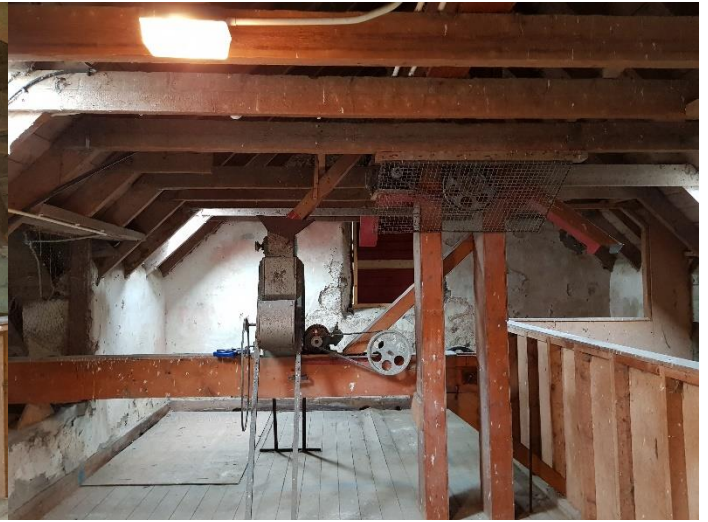
Figure 21: The grain conveyor to the byre, and the west end of the gallery
