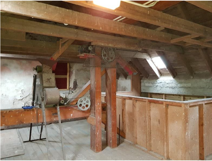
Figure 20: The top of the granary hopper on the right. Note, the grain conveyor on the left distributing grain to the byre
