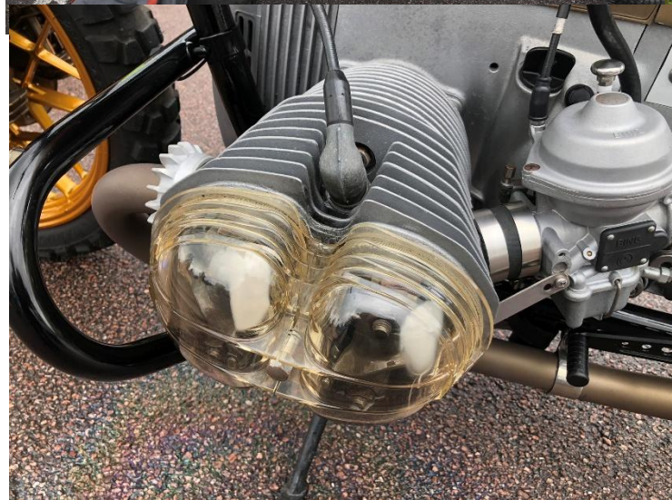
This BMW special has transparent rocker covers.
