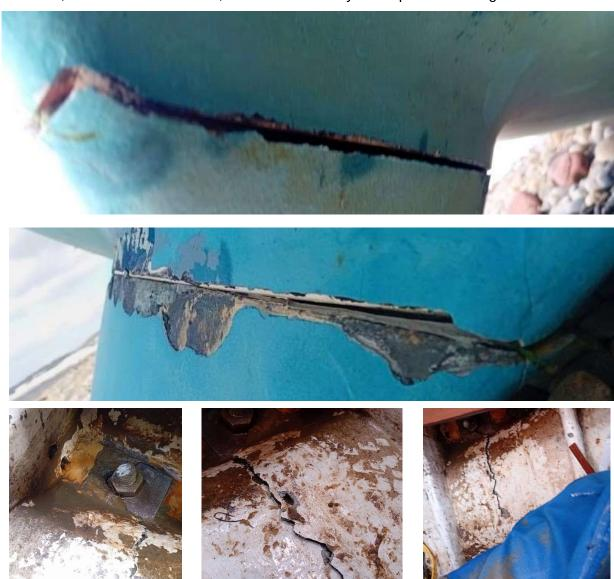
Most of the damage is to the keel, it has come away from the hull as you can see and there are cracked areas inside around the keel bolts. The mast of this boat is keel stepped so we won't know much more until closer examination once the boat is on dry land, which hopefully will be by the weekend
