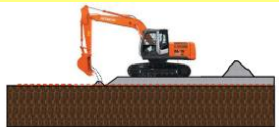
Fig 7.2 Dropped on to geogrid
