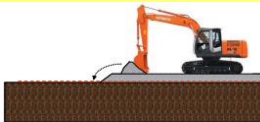
Fig 7.1 Pushed forward from stockpile
